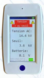
DTI interface with information, repeater mode and voltmeter.
