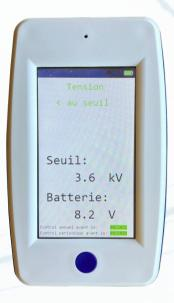
DTI interface with information and repeater mode. Indication of the detection threshold programmed in the device as well as the voltage value of its battery. Indication of the date of the next annual check (recommended) Indication of the date of the next periodic inspection (mandatory) Audible signaling with indication of voltage overshoot of the threshold voltage. (left image below threshold, right image above threshold)
